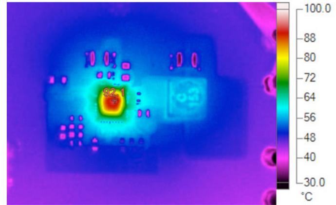
Conditions: 100V<sub>IN</sub>, 5V<sub>OUT</sub> at 2.3A<sub>OUT</sub>
