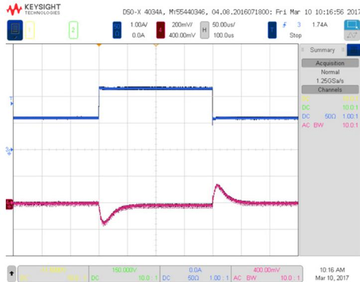
Figure 6. Transient Response Waveform at 48V<sub>IN</sub>, 5V<sub>OUT</sub> and 1.1A<sub>OUT</sub> to 2.3A<sub>OUT</sub> to 1.1A<sub>OUT</sub> (1A, 200mV, 50μs/DIV, 20MHz Bandwidth)
