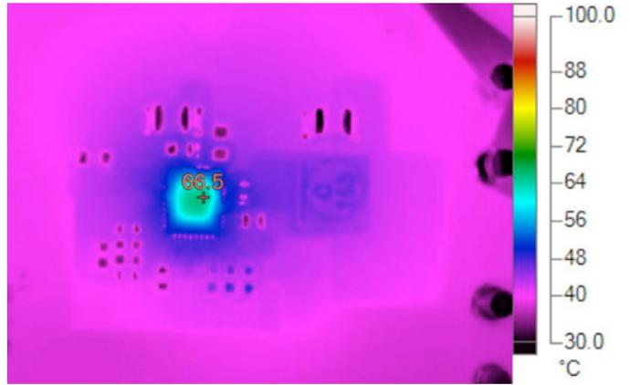
Conditions: 24V<sub>IN</sub>, 5V<sub>OUT</sub> at 2.3A<sub>OUT</sub>
