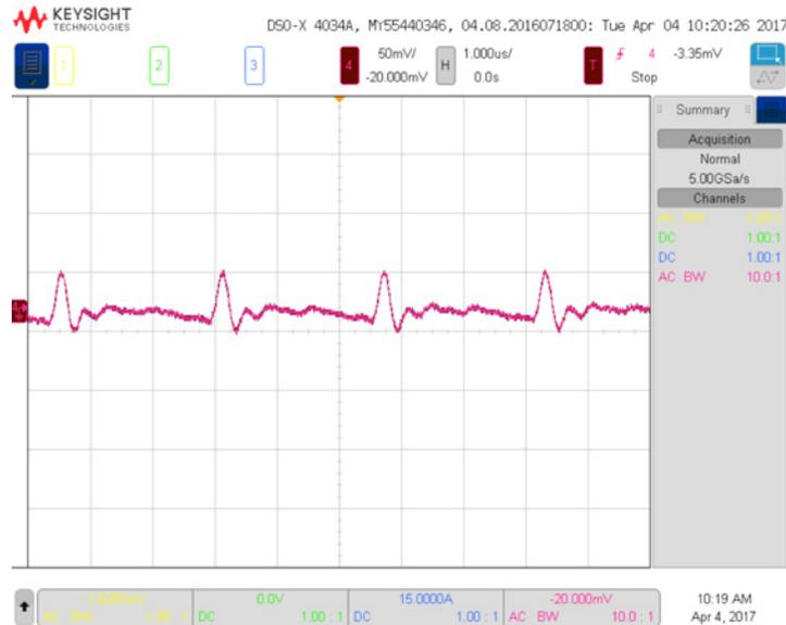
Figure 5. Output Ripple at 100V<sub>IN</sub>, 5V<sub>OUT</sub> and 2.3A<sub>OUT</sub> (50mV, 500ns/DIV, 20MHz Bandwidth)
