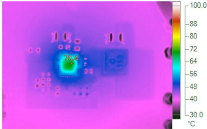
Conditions: 48V<sub>IN</sub>, 5V<sub>OUT</sub> at 2.3A<sub>OUT</sub>
