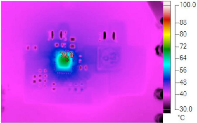
Conditions: 12V<sub>IN</sub>, 5V<sub>OUT</sub> at 2.3A<sub>OUT</sub>
