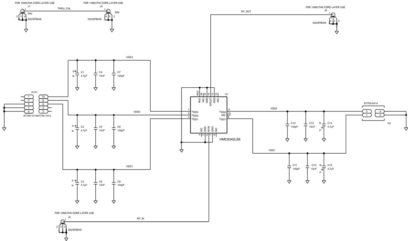
Figure 4. EV1HMC8342LS6 Schematic
