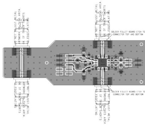
Figure 5. EV1HMC8342LS6 Silk Screen and Metal 1, Top Side
