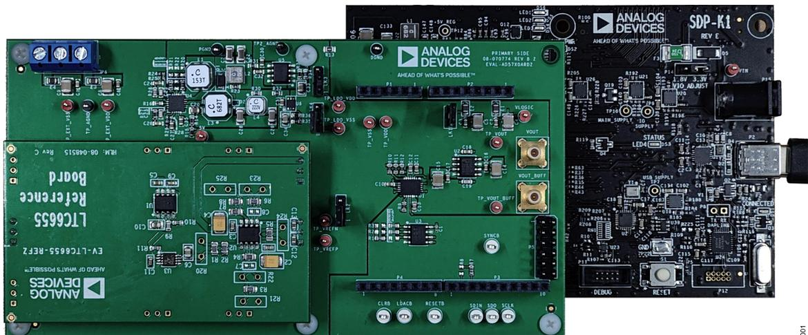
Figure 1. The EVAL-AD5780ARDZ Connected to the SDP-K1 Controller Board
