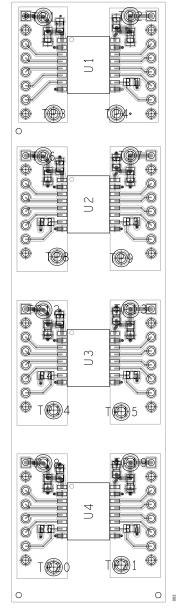
Figure 3. EVAL-ADuM34XEEBZ Component Side, Layer 1
