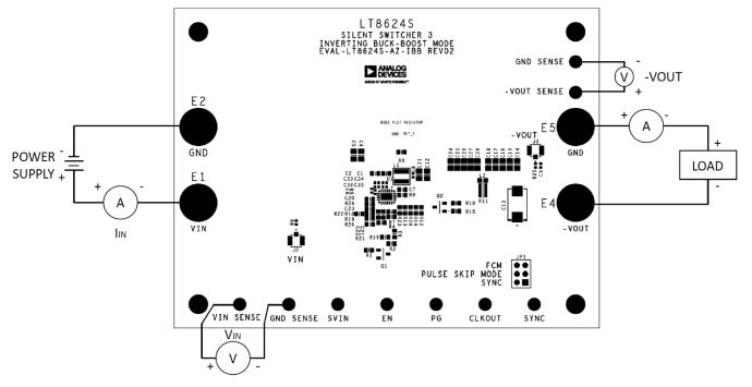
Figure 8. Board Test Setup
