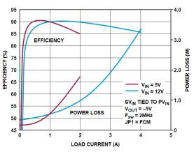
Figure 1. Efficiency vs. Load Current (Input from V<sub>IN</sub> Terminal)
