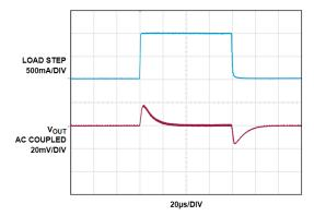
Figure 6. Load Transient Response from 0A to 1A to 0A with a 1A/ $\mu$ s Slew Rate, V<sub>IN</sub> = 5V, V<sub>OUT</sub> = -5V. V<sub>OUT</sub> Measured Through J3
