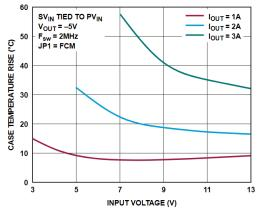
Figure 2. Case Temperature Rise vs. V<sub>IN</sub>
