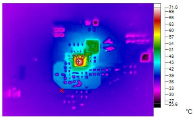
Figure 7. Thermal Performance at  $V_{IN}$  = 5V, SV<sub>IN</sub> tied to PV<sub>IN</sub>,  $V_{OUT}$  = -5V,  $I_{OUT}$  = 2A,  $T_A$  = 25°C
