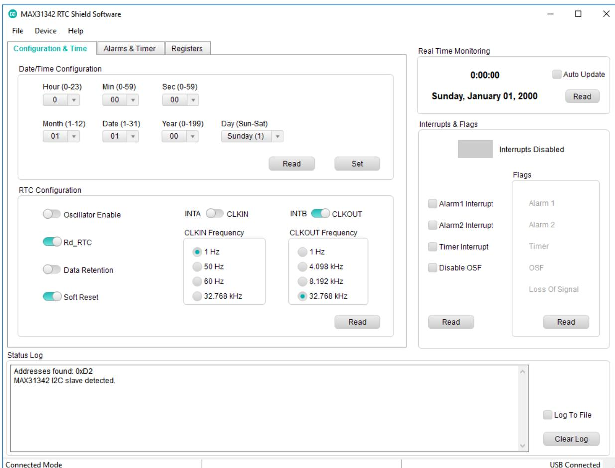
Figure 3. Configuration & Time tab.
