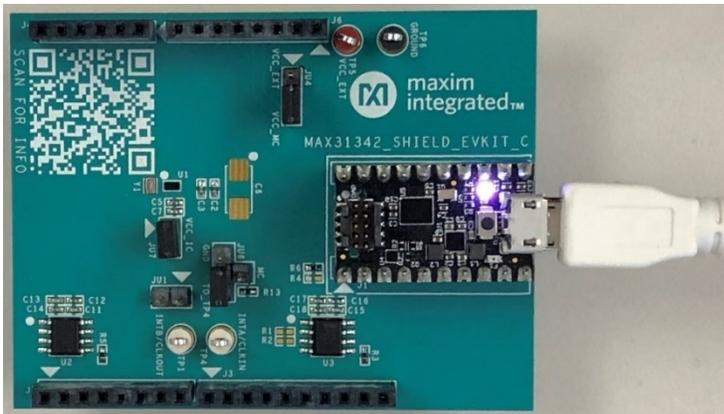
Figure 1. MAX31342 Shield with MAX32625PICO.
