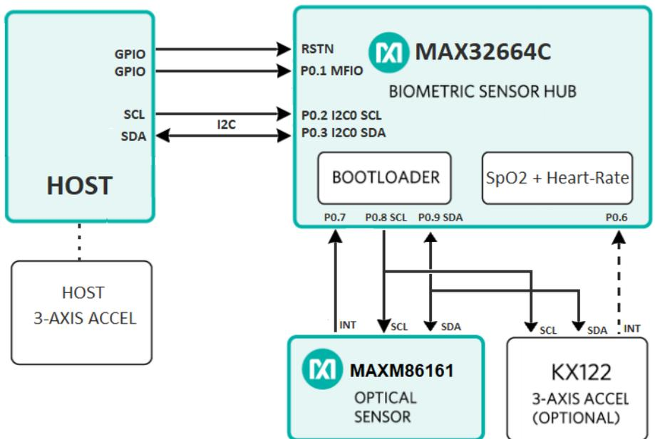
Figure 2. Architecture diagram for health-sensing applications using an I<sup>2</sup>C interface to communicate with the sensor (such as the MAXM86161).
