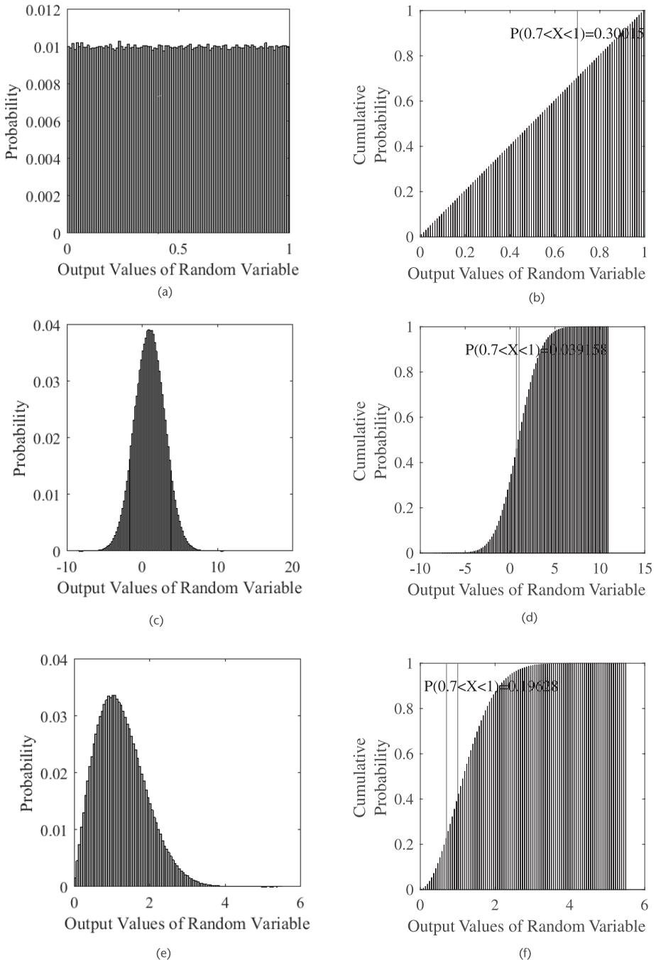
**Figure 3.5** Various cumulative distribution functions and associated probability density functions. (a) Uniform PDF, (b) uniform CDF, (c) Gaussian PDF, (d) Gaussian CDF, (e) Rayleigh PDF, and (f) Rayleigh CDF.
