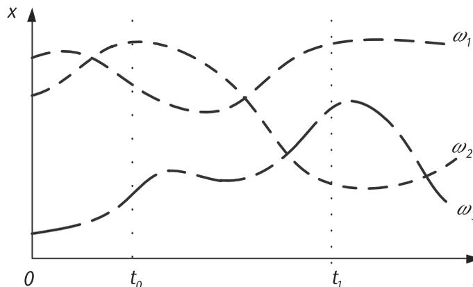
**Figure 3.6** Illustration of a random process  $X(t, \omega)$ .
