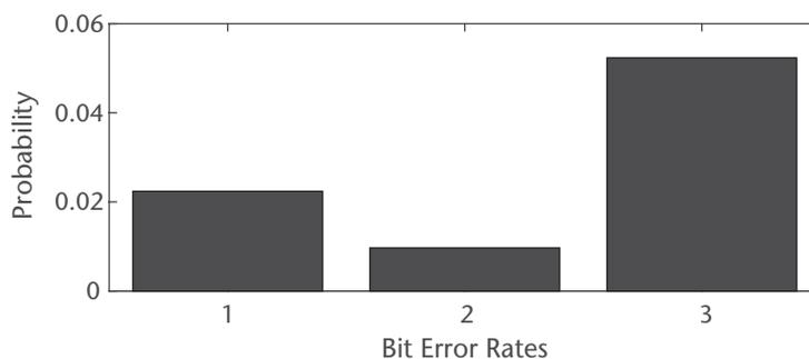
**Figure 3.3** Binary channel error probabilities when the probability for a zero being received uncorrupted is 0.95 and the probability for a one being received uncorrupted is 0.99. Note that the transmission consists of 40% ones and 60% zeros. 1 = Total, 2 = one transmitted, 3 = zero transmitted.
