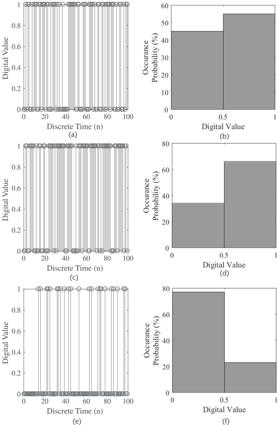
**Figure 3.1** Stem plots and histograms of three binary transmissions that each possess different probabilities of ones and zeros being produced. (a) Binary signal (50% ones, 50% zeros), (b) histogram (50% ones, 50% zeros), (c) binary signal (60% ones, 40% zeros), (d) histogram (60% ones, 40% zeros), (e) binary signal (20% ones, 80% zeros), and (f) histogram (20% ones, 80% zeros).
