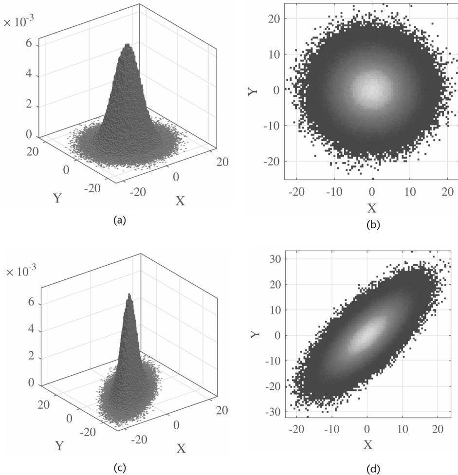
**Figure 3.8** Several examples of correlated and uncorrelated bivariate Gaussian densities. (a) Uncorrelated bivariate Gaussian (3-D view), (b) uncorrelated bivariate Gaussian (top-down view), (c) correlated bivariate Gaussian (3-D view), and (d) correlated bivariate Gaussian (top-down view).
