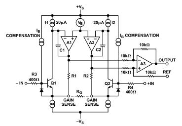
Figure 3-7. A simplified schematic of the AD620.
