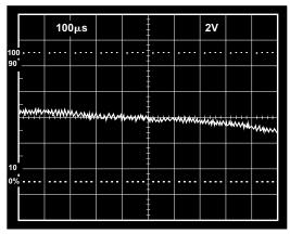
Figure 3-18. AD621 gain nonlinearity ( $G = 10, R_L = 10 \ k\Omega$ , vertical scale: 100  $\mu$ V/div = 100 ppm/div, horizontal scale 2 V/div).
