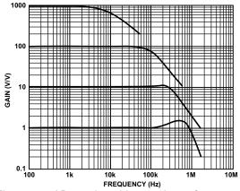
Figure 3-8. AD620 closed-loop gain vs. frequency.
