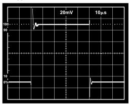
Figure 3-19. Small signal pulse response of the AD621 (G = 10,  $R_L = 2 k\Omega$ ,  $C_L = 100 pF$ ).
