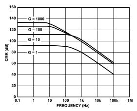
Figure 3-12. AD622 CMR vs. frequency ((RTI) 0 to 1  $k\Omega$  source imbalance).
