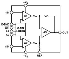
Figure 3-52. AD8250 and AD8251 simplified schematic.
