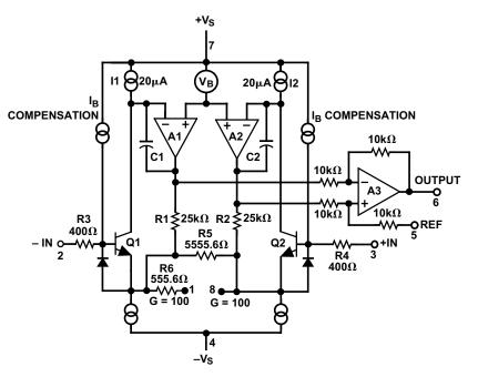
Figure 3-15. A simplified schematic of the AD621.
