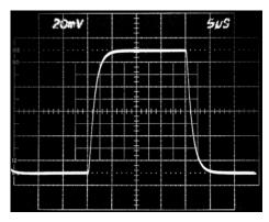
Figure 3-46. AD623 small signal pulse response (G = 10,  $R_L$  = 10 k $\Omega$ ,  $C_L$  = 100 pF).
