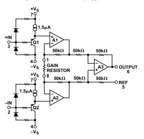
Figure 3-42. AD623 simplified schematic.
