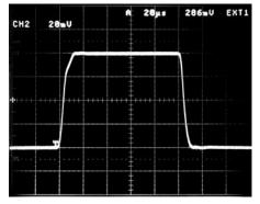
Figure 3-51. Small signal pulse response of the AD627 ( $V_S = \pm 5 V$ , G = +10,  $R_L = 20 k\Omega$ ,  $C_L = 50 pF$ , 20 µs/horizontal division, 20 mV/vertical division).
