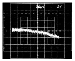
Figure 3-45. AD623 gain nonlinearity (G = -10, 50 ppm/div).
