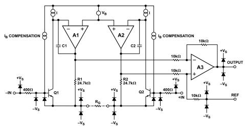
Figure 3-1. AD8221 simplified schematic.
