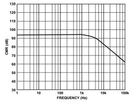
Figure 3-40. AD8225 CMR vs. frequency.
