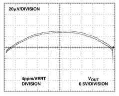
Figure 3-50. AD627 gain nonlinearity  $(V_S = \pm 2.5 V, G = 5, 4 \text{ ppm/vertical division}).$
