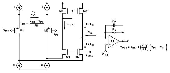
Figure 3-33. AD8553 simplified schematic.
