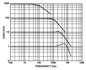
Figure 3-14. AD622 closed-loop gain vs. frequency.
