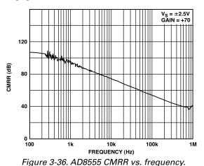
Figures 3-36 and 3-37 show the AD8555's CMRR vs. frequency and its closed-loop gain vs. frequency.
