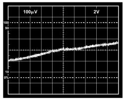
Figure 3-10. AD620 gain nonlinearity (G = 100, R<sub>L</sub> = 10 k $\Omega$ , vertical scale: 100  $\mu$ V = 10 ppm, horizontal scale: 2 V/div).
