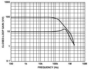
Figure 3-17. AD621 closed-loop gain vs. frequency.
