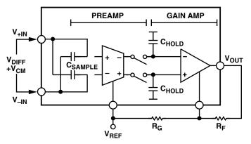
Figure 3-23. The AD8230 in Phase A sampling phase. The differential component of the input signal is stored on sampling capacitors,  $C_{SAMPLE}$ . The gain amp conditions the signal stored on the hold capacitors,  $C_{HOLD}$ . Gain is set with the  $R_G$  and  $R_F$  resistors.
