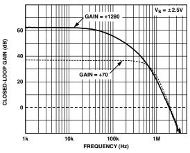
Figure 3-37. AD8555 closed-loop gain vs. frequency measured at output pin.
