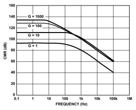
Figure 3-9. AD620 CMR vs. frequency.
