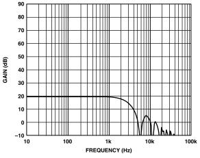
Figure 3-31. Gain vs. frequency, G = 10.
