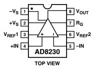
Figure 3-22. AD8230 connection diagram.
