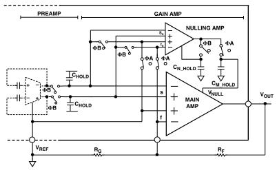
Figure 3-26. Detailed schematic of the gain amp during Phase A. The main amp conditions the signal held on the hold capacitors,  $C_{HOLD}$ . The nulling amplifier forces the inputs of the main amp to be equal by injecting a correction voltage into the  $V_{NULL}$  port, removing the offset of the main amp. The correction voltage is stored on  $C_{M \ HOLD}$ .
