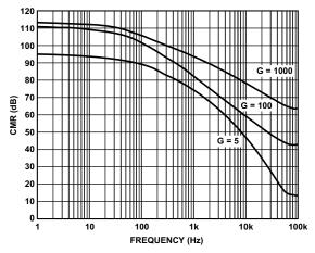
Figure 3-48. AD627 CMR vs. frequency.
