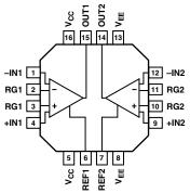
Figure 3-5. AD8222 connection diagram.
