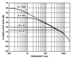
Figure 3-49. AD627 closed-loop gain vs. frequency.
