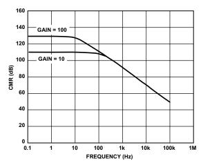
Figure 3-16. AD621 CMR vs. frequency.
