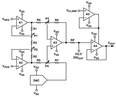
Figure 3-35. AD8555 simplified schematic.
