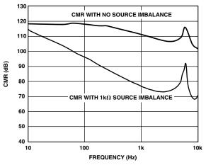
Figure 3-30. Common-mode rejection vs. frequency.
