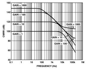
Figure 3-3. CMRR vs. frequency (RTI) of the AD8221.
