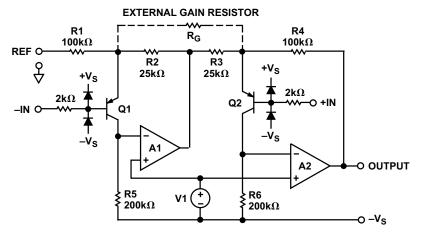
Figure 3-47. AD627 simplified schematic.
