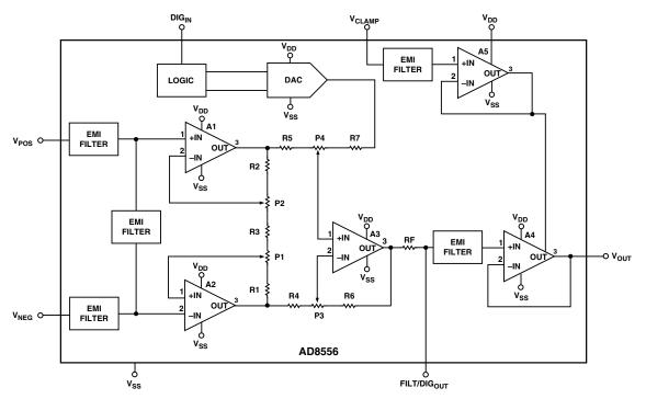
Figure 3-38. AD8556 block diagram showing EMI/RFI built-in filters.
