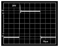
Figure 3-11. Small signal pulse response of the AD620 (G = 10,  $R_L$ = 2 k $\Omega$ ,  $C_L$  = 100 pF).
