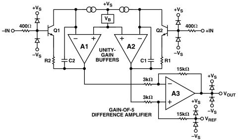
Figure 3-39. AD8225 simplified schematic.
