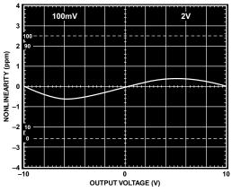
Figure 3-41. AD8225 gain nonlinearity.
