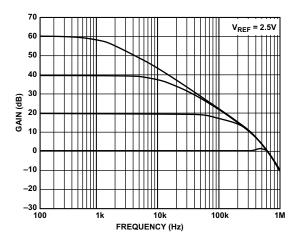
*Figure 3-43. AD623 closed-loop gain vs. frequency.*
