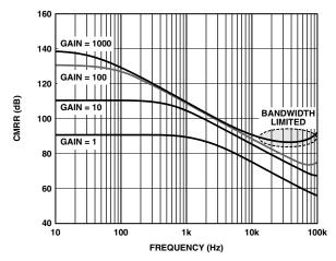
Figure 3-21. Typical AD8220 CMRR vs. frequency.
