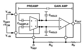
Figure 3-24. In Phase B, the differential signal is transferred to the hold capacitors, refreshing the value stored on  $C_{HOLD}$ . The gain amp continues to condition the signal stored on the hold capacitors,  $C_{HOLD}$ .
