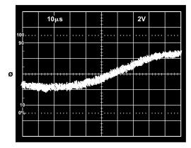
Figure 3-13. AD622 Gain nonlinearity (G = 1,  $R_L$  = 10 k $\Omega$ , vertical scale: 20  $\mu$ V = 2 ppm).
