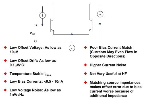
Figure 2: A Bias Current Compensated Bipolar Input Stage
