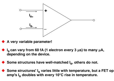
• Some structures have I<sub>B</sub> which may flow in either direction.
